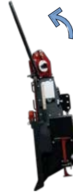
5.2.3 Tilt the winch away from the tractor
