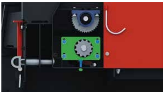
733 Tightening the first drive chain
