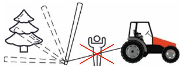
25.4 Obstacles can cause the timber to tip up or sideways
