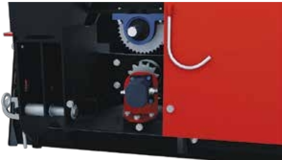
732 Tightening the pump chain
