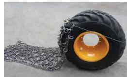
5. Check the center of the chain pattern follows the centre of the tire pattern
