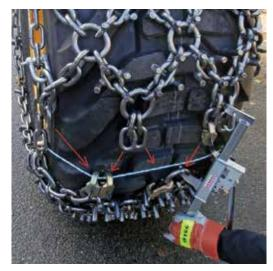
7. Connect the mesh (use the additional links enclosed if necessary)
