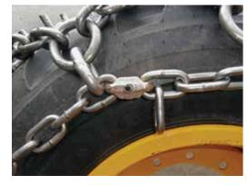
10. If fitted, adjust tightening rail
