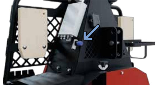
6.3.1 Speed control for Pullmatic
