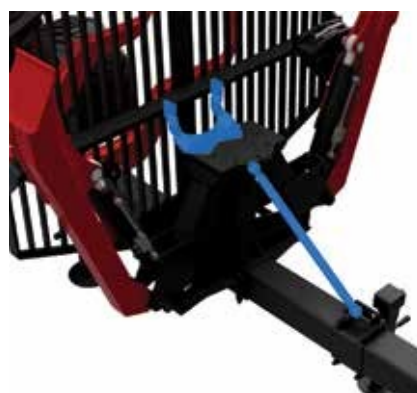
6.10.1 Attaching the 3-point frame
