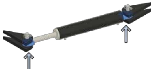
10.3.2 Swivel cylinders for bogie Both sides of the trailer
