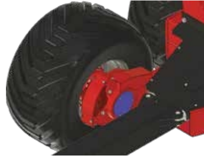
10.1.1 Cover for access to hub motor bolts
