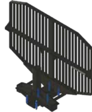
5.6.1 Bolts for attaching the grid
