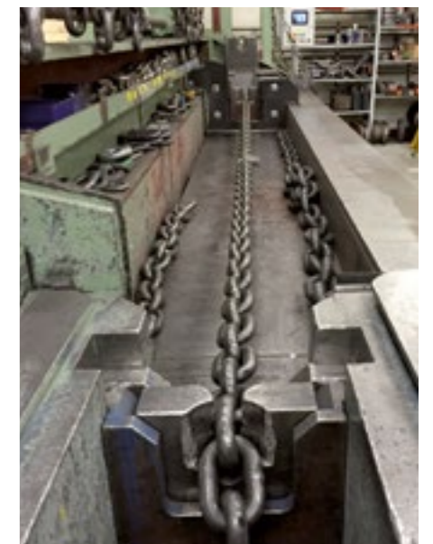
Test Station CT 200
