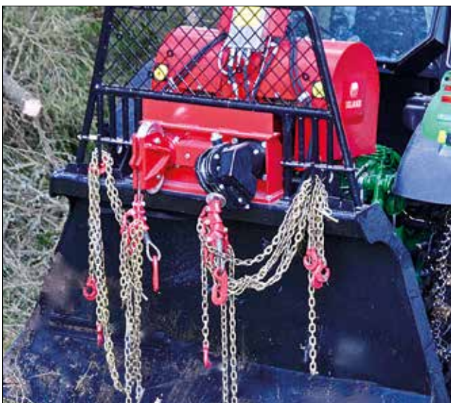
Black port shows pullmatic which makes the work of "pulling" the wire out a breeze
