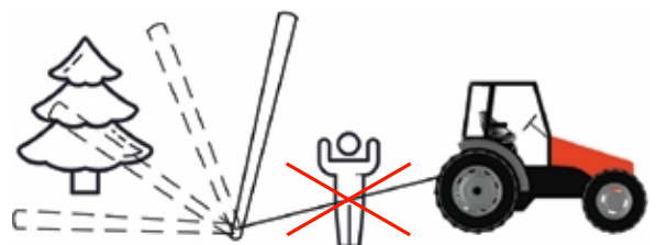
15.4 Obstacles can cause the timber to tip up or sideways.
