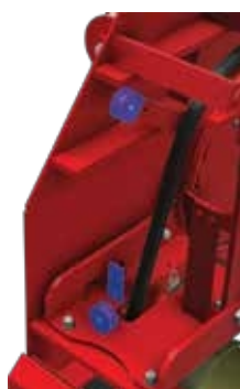
5.6.2 Attaching the rope to the cleat
