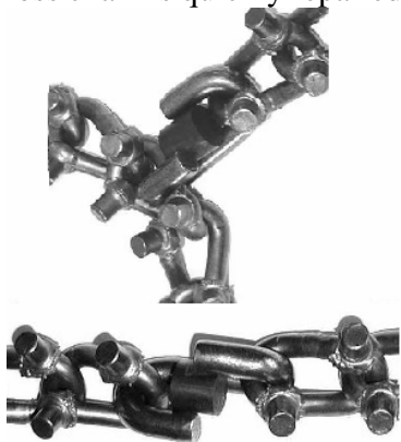
Repair With S-link above. Repair with Z-link below.
