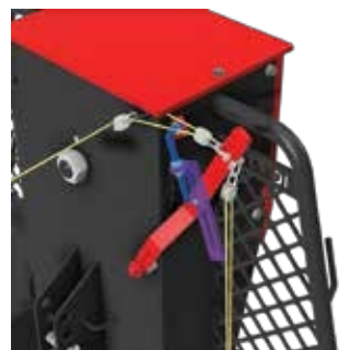
7.9.1 Rod for adjusting overlap between the brake shoe and brake
