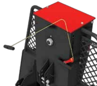
5.2 .1 Rope for pawl brake on 42 and 52
